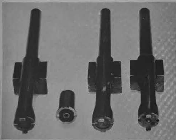
Breech-bolts for Henry (left) and Model '66 R. F. and C. F. (right) Note Auxiliary Chamber patented by O. F. Winchester Courtesy of Winchester Repeating Arms Company
