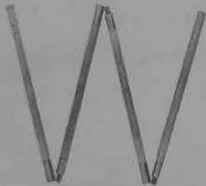
Jointed Wiping Rod for Henry Rifle Coll's Manufacturing Company
